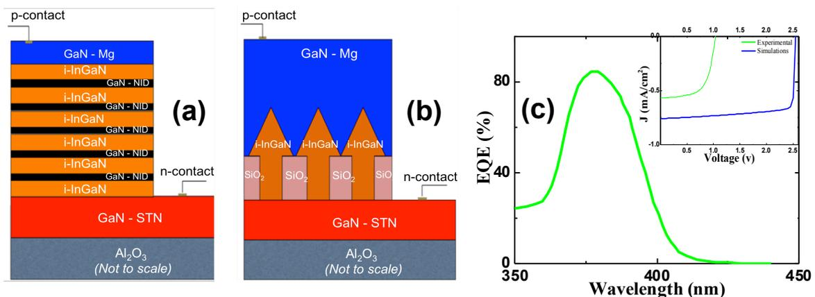
Figure 1: (a) Semibulk InGaN, (b) Nano-structured InGaN, (c) EQE and  $J$ - $V$  results for semibulk  $\text{In}_{0.08}\text{Ga}_{0.92}\text{N}$  PV cell.
